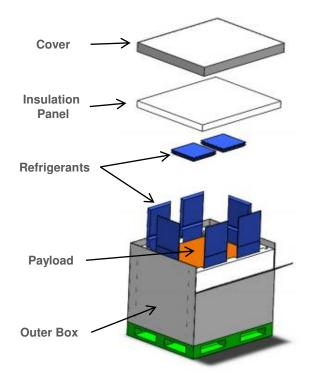
Cryopak also specializes in parcel-sized insulated containers. Offered in both single-use and reusable options, they are ideal for shipping smaller quantities while preventing product exposure to freezing or excessively high temperatures.
